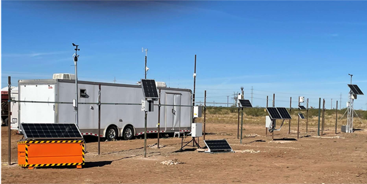
Figure 3-1. Field intercomparison site used in Project Astra to evaluate four methane sensing systems.
